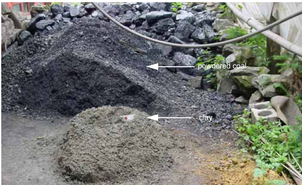
Figure 8. Powdered coal, which is one third of the price of lumps of coal, is mixed with clay to form briquettes so that air spaces are present in the fire to allow the coal to burn. The clay acts as an adhesive to form lumps of a mixture of coal powder and clay. The air can enter between the lumps in the fire thus allowing the coal to burn.
